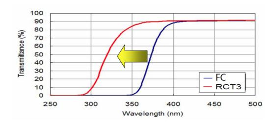
RCT3 has high transmittance at UV region compared to FC
